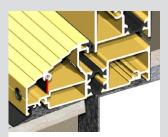
We have designed and tested hinged doors that open in and doors that open out with custom thermally broken sills that keep water out.
